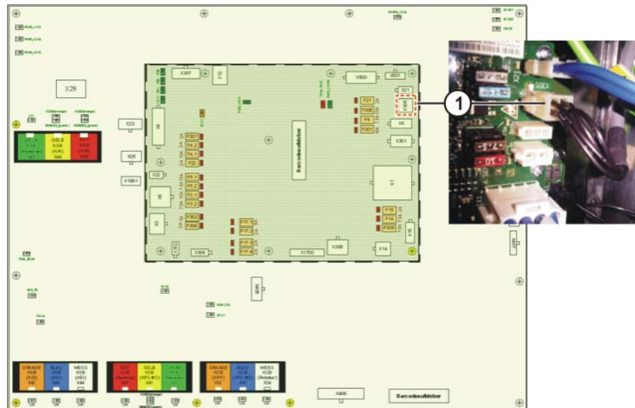
Fig. 8-1: Battery discharge protection X305
